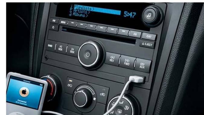
The **NEW USB** port, available in LT and SS models, connects the jump drive and offers complete functionality through HHR's stereo system. Flip through your tunes using the available steering wheel-mounted audio controls while the radio displays all of your playlist information from your MP3 player or select iPod<sup>®10</sup> models.
