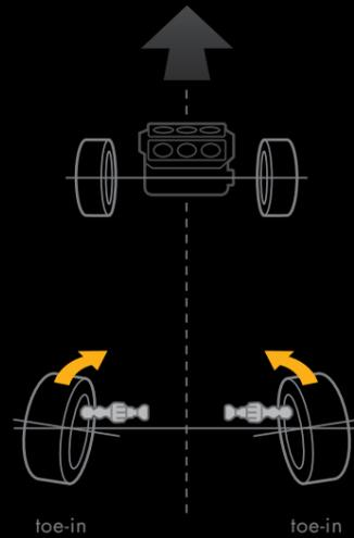
As a turn begins, the inner rear wheel adjusts to help direct the vehicle.
