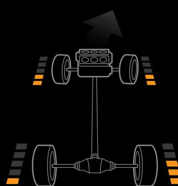
For increased stability during lane changes, the SH-AWD system transfers power to the inside rear wheel.
