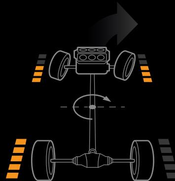
When cornering on dry surfaces, up to 70% of the torque is distributed to the rear. Torque vectoring allows up to 100% of the power to distribute to the outside rear wheel, improving control and helping rotate the TLX through the turn.
