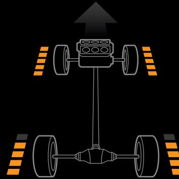
As weight shifts to the rear of the TLX during hard acceleration, the SH-AWD system transfers up to 44% of the power to the rear wheels to take advantage of available traction.
