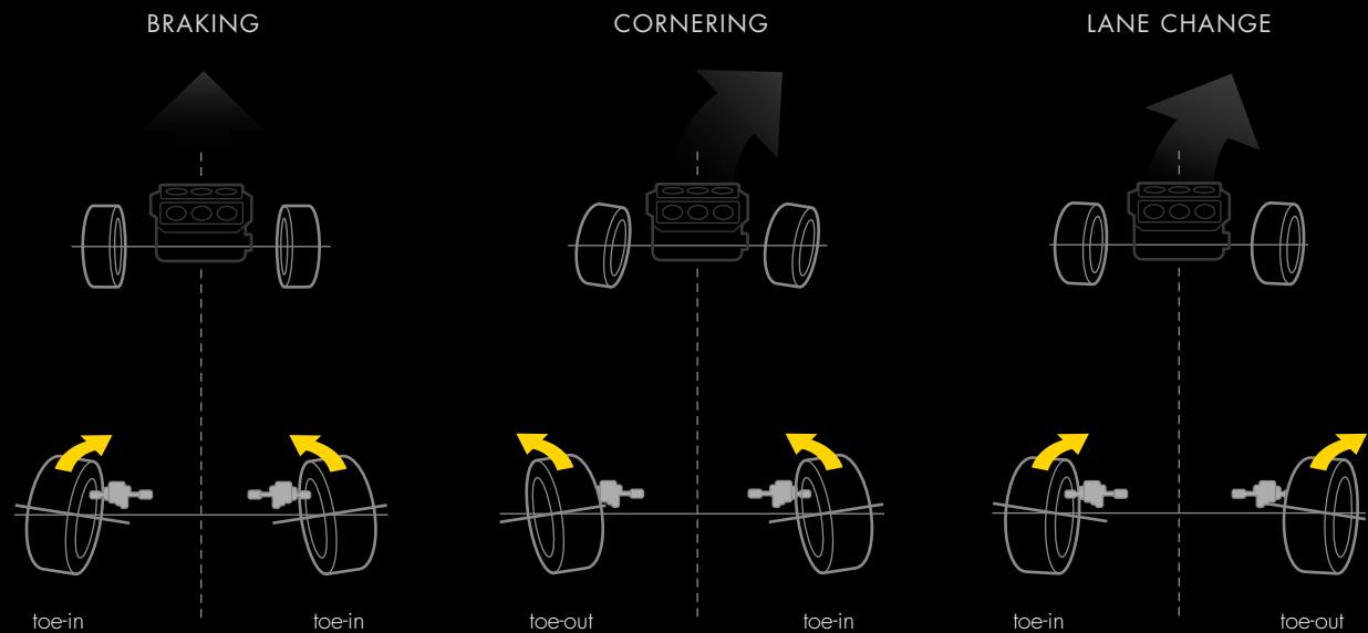
While braking, each rear wheel adjusts inward, increasing stability.
