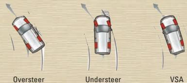
**Vehicle Stability Assist™ (VSA®)** system helps sense oversteer or understeer and brakes individual wheels and/or reduces engine power to help keep you on your intended course.
