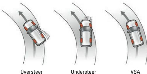
**Vehicle Stability Assist (VSA).**<sup>†</sup> Standard on every Element, VSA employs sensors to monitor for oversteer or understeer. It adjusts brake pressure at each wheel and/or reduces engine power to help restore the vehicle to its intended path.
