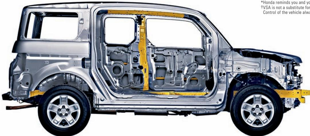
**Unit-body construction.** Incorporating front and rear crumple zones, the Element's chassis is designed to minimize the amount of crash energy entering the passenger compartment. Side-impact door beams help provide enhanced structural protection and help reduce the likelihood of cabin intrusion.
