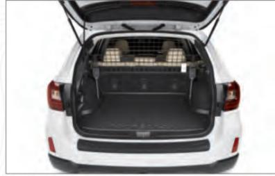
**Compartment Separator.** Helps to separate cargo from the passenger area.
