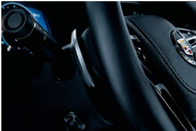
Dual-side paddle controls located behind the steering wheel provide regeneration on demand, putting energy back into your battery while simultaneously slowing you down. This technology is something you can only truly appreciate when you experience it from behind the wheel – especially in slow-and-go traffic where exclusive Regen on Demand™ gives you the comfort of one-pedal driving.
