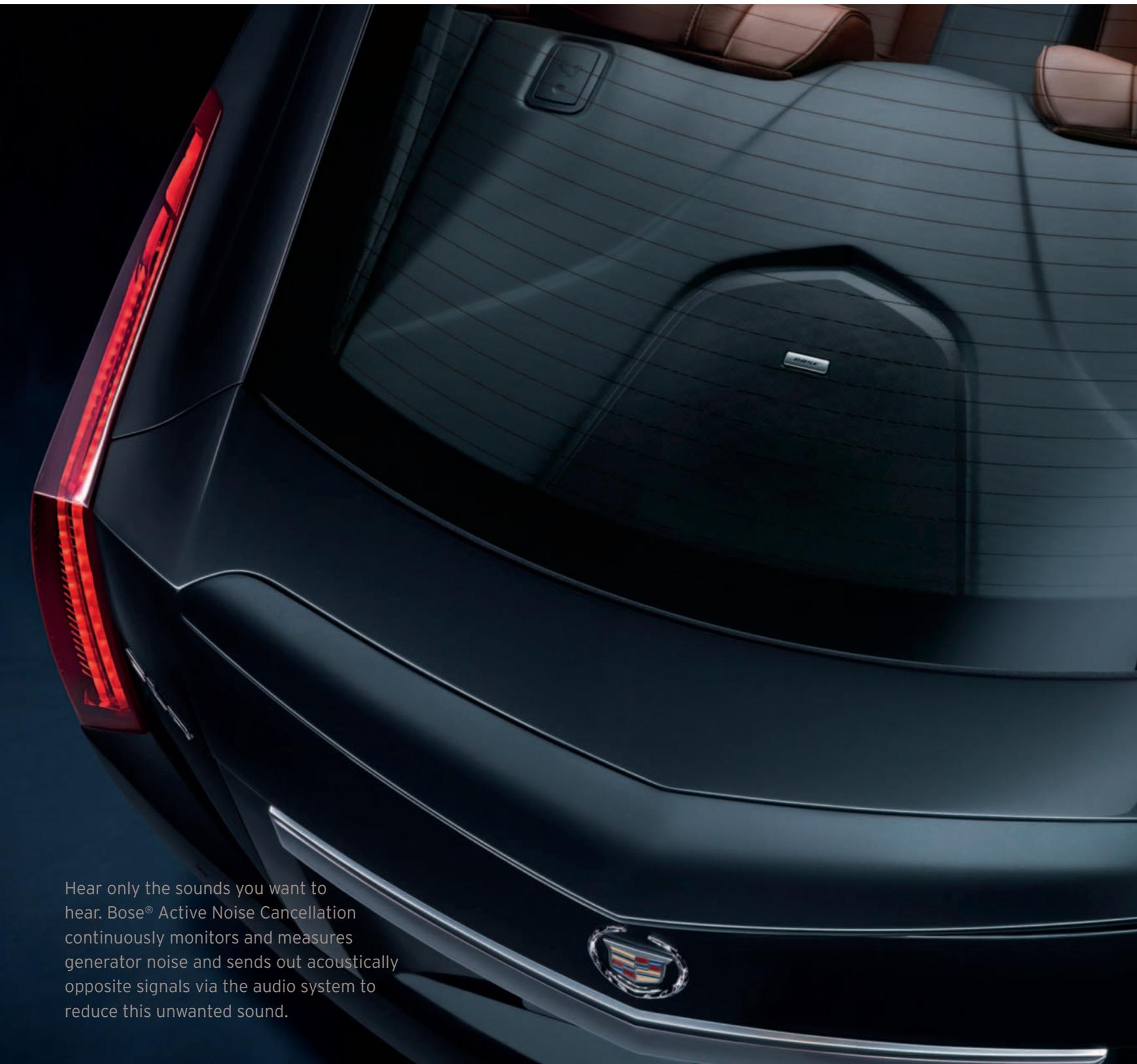
Hear only the sounds you want to hear. Bose® Active Noise Cancellation continuously monitors and measures generator noise and sends out acoustically opposite signals via the audio system to reduce this unwanted sound.
