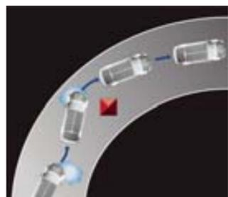
**Vehicle Dynamics Control** This stability system helps keep you on your intended path by measuring variables such as steering input, braking and vehicle angle. Sensing any slide that causes the vehicle to deviate from your intended course, VDC applies individual brakes and/or reduces engine power to counteract the slide and help keep you safely in control.
