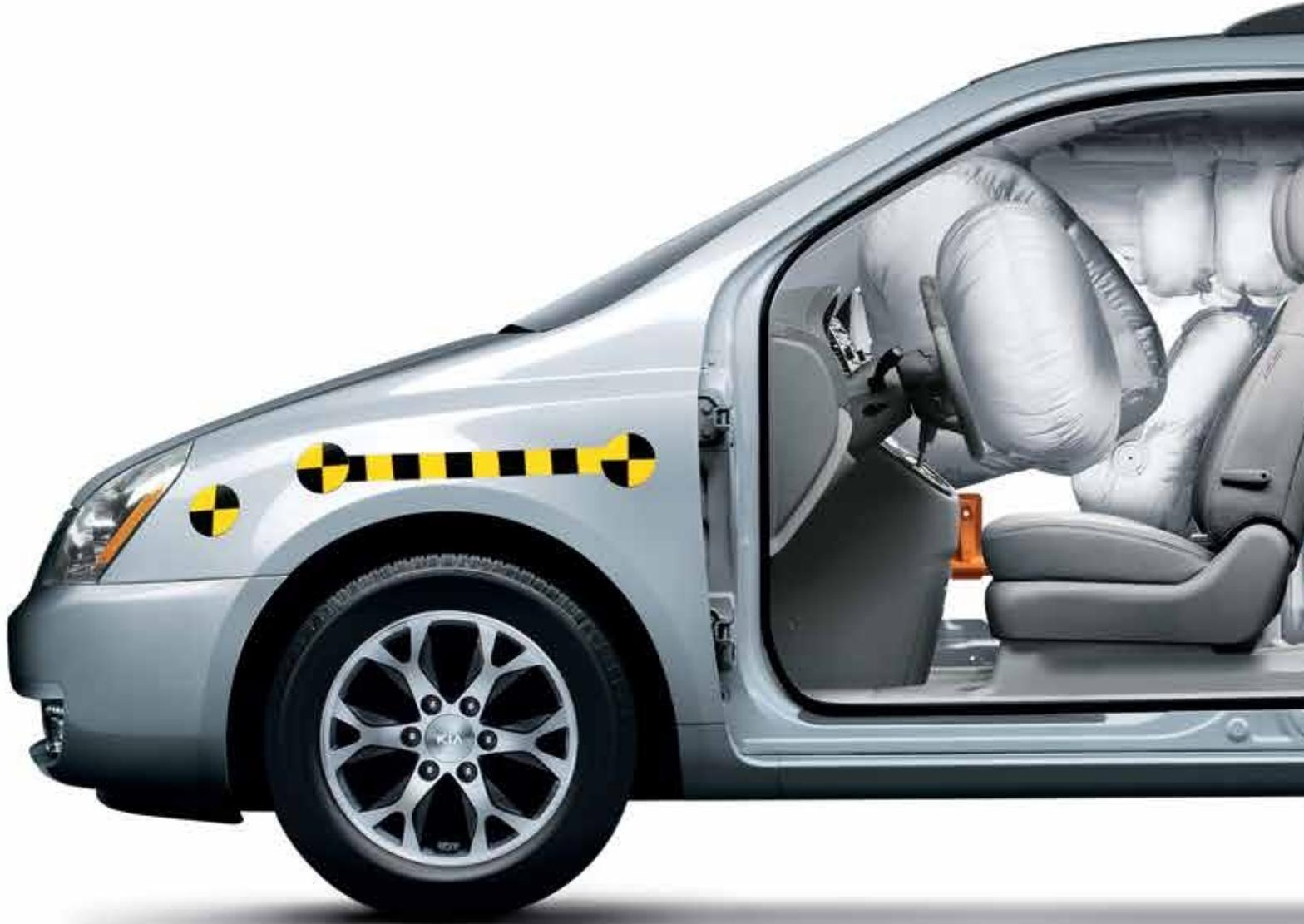
Sedona is equipped with a range of passive safety systems.<sup>†</sup> Six airbags placed throughout the cabin are designed to help protect occupants in certain collisions. They include dual front advanced, dual front seat-mounted side, and full-length side-curtain airbags. The advanced front airbag system monitors the severity of a frontal impact, the presence of a front passenger and seat-belt use, and then controls airbag inflation accordingly.<sup>5</sup>
