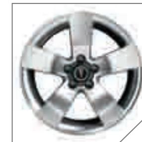
C – 19" machine-faced aluminum (C)
