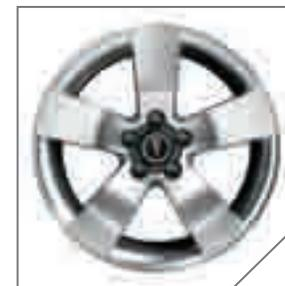
C – 19" machine-faced aluminum (C)
