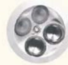
**Four-valve cylinder head.** All L-Series engines are designed with two intake and two exhaust valves per cylinder. This enables them to breathe more freely for better combustion than two-valve designs. This translates into more torque, better acceleration and reduced emissions.
