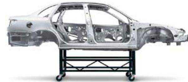
**L-Series modified spaceframe.** If automobile safety had a heart, this would certainly be it. A steel structure that encases the passenger compartment and is designed with front and rear crumple zones to help absorb the energy from a crash. There's also a great side benefit to the solid design—fewer squeaks and rattles down the road.
