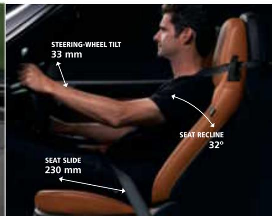
An enhanced driving position and superb support are provided by the MX-5 Miata's high-bolstered driver's seat. Its all-new design accommodates 95% of all male drivers via a refined design, wider range of adjustments and a tilt-adjustable steering wheel. In addition, redesigned and repositioned foot pedals help instill driver confidence and facilitate "heel-and-toe" shifting.
