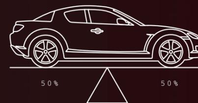
WEIGHT DISTRIBUTION significantly impacts a sports car's stability and handling. So the Mazda RX-8 is engineered to maintain an approximate 50:50 weight distribution, front to rear, regardless of passenger load. The end result is a remarkably agile, well-balanced design.
