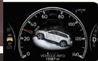
**CAPABILITY** See the current settings for your available Quadra-Lift® Air Suspension System and steering-wheel position. You can also see how your available Selec-Terrain® system is functioning via perspective visuals.
