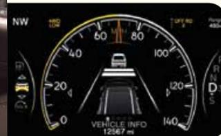
**VEHICLE INFO** When the available Adaptive Cruise Control (ACC)<sup>13</sup> with Stop senses a vehicle ahead, it will apply limited braking or acceleration automatically to maintain a pre-set following distance, while matching the speed of the vehicle ahead.
