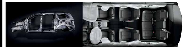
**STRATEGICALLY PLACED HIGH-STRENGTH STEEL.** Town & Country architecture includes dual-phase, high-strength and hot-stamped steel, resulting in a strong safety cage that contributes to overall vehicle-impact performance.
