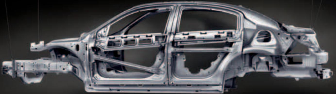
Specifically designed front and rear crumple zones help absorb energy and redirect it away from passengers, helping to reduce the risk of injury in the event of a collision.
