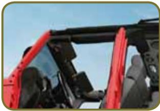
The Sunrider® Soft Top lets you quickly get cover or let the sun shine in without having to fold back the entire top. The opening is huge: 55x30 inches in Wrangler and a massive 55x60 inches in Wrangler Unlimited (extends all the way over the rear occupants). All soft tops use a unique three-ply sailcloth fabric that helps to reflect road sounds, absorb wind noise, prevent buffeting and enhance overall insulation. The soft tops are also easy to fold and tuck away.
