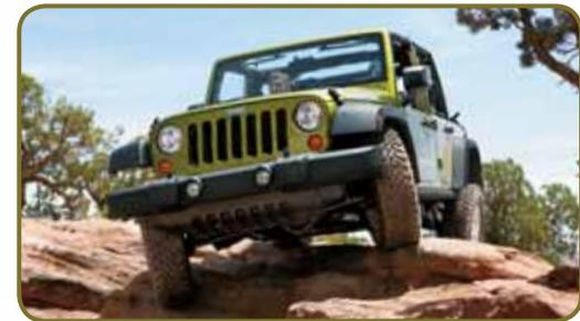
When activated the standard electronic sway bar disconnect automatically disengages its front sway bar when driving under 18 mph in 4WD 4LO mode.
