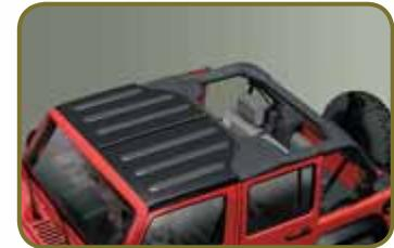
The available Freedom Top three-piece modular hardtop allows for easier handling and storage by separating into three manageable pieces. Without the two front panels, the back of the hardtop is now much easier for two adults to remove. The available Authentic Jeep® Accessories by Mopar Freedom Top Carrier allows the panels to be conveniently carried on the spare tire.
