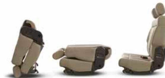
The Fold and Tumble rear seat is standard on Wrangler two-door models. Wrangler four-door models come with split-folding rear seat.
