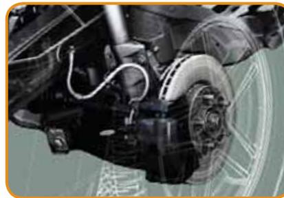
Front-wheel-drive Compass still benefits from a MacPherson strut/multilink suspension with the traction and agility such a combination provides.
