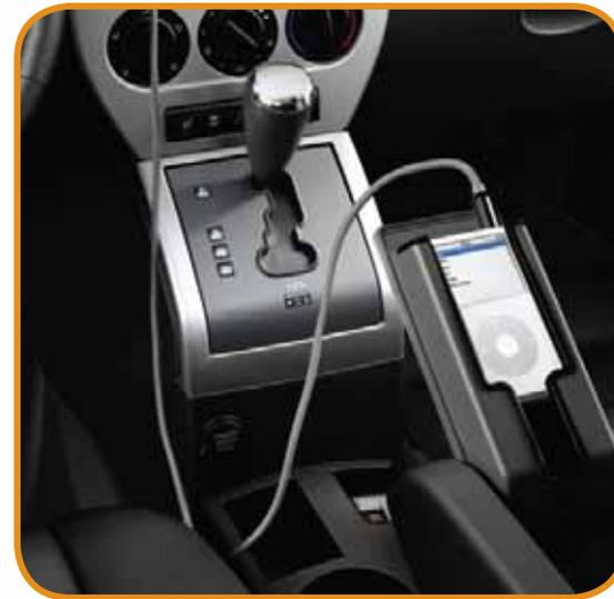
The standard center console features a sliding storage armrest with a rubber-lined lid panel that flips forward to cradle an MP3 player or mobile phone — and snugly at that.
