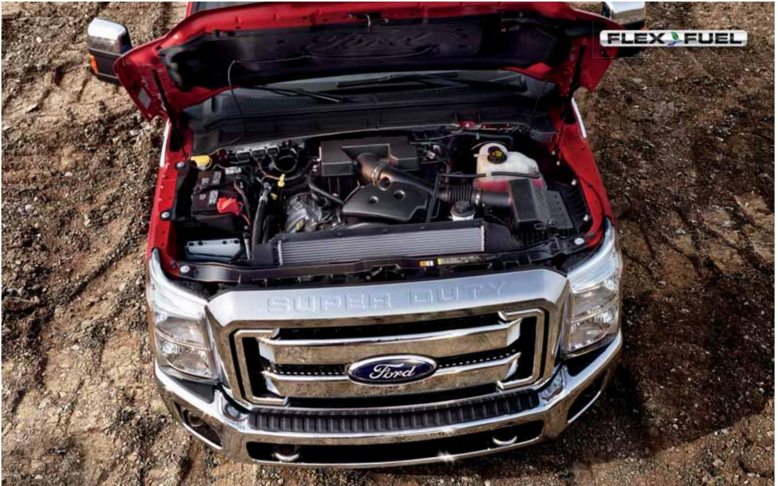
**Produces significant low-rpm torque.** The stiff SOHC valvetrain with roller-rocker shafts also enables an intake- and exhaust-port layout that optimizes airflow.
