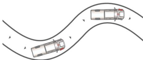
**Masters challenging moments.** Our exclusive AdvanceTrac® with RSC® (Roll Stability Control™) is the only electronic stability control system in the class that utilizes 2 gyroscopic sensors to help keep all 4 wheels firmly planted.<sup>3</sup> It automatically helps avoid skidding and fishtailing, and is particularly beneficial in inclement weather.
