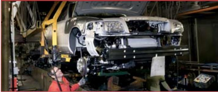
The Police Interceptor's body is secured to a separate, ultra-sturdy frame – composed of hydroformed steel – for increased structural rigidity and durability, outstanding ride quality and impressive road-noise reduction. While the Crown Victoria is built in the **body-on-frame** manner of most trucks, both the Charger and Impala simply utilize unibody construction with no separate frame.
