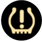
TPMS can warn of underinflation and overinflation that can damage tires or cause a blowout. An active pressure sensor with a radio transmitter is mounted inside the tire on each wheel (except the spare). A receiver in the Crown Victoria Police Interceptor monitors each transmitter, and if tire pressure isn't within specified limits, a warning light with an audible tone will activate.
