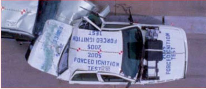
Ford Crown Victoria Police Interceptor is the only police pursuit sedan on the market designed to meet **75-mph rear-end crash tests** without a fuel tank puncture. Ford is also the only vehicle manufacturer to publish results for a 75-mph test – the same can't be said for Charger or Impala.
