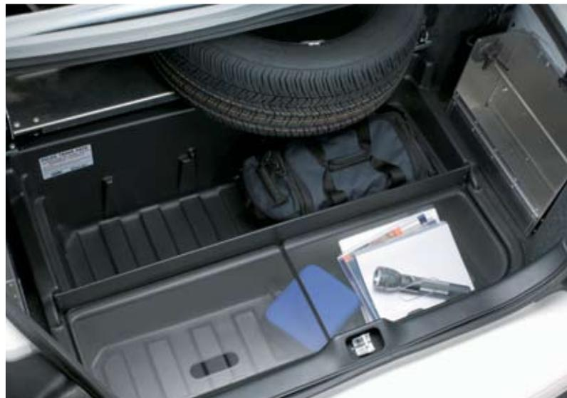
**CAUTION:** Do not place stiff or sharp objects in the trunk that could be pushed forward into the fuel tank in a high-speed rear impact.
