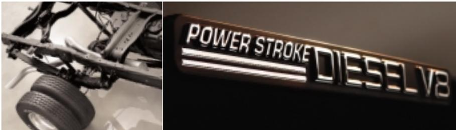
Steel ladder-type frame construction for strength. Multi-leaf rear springs for solid support. Front and rear stabilizer bars. 16" wheels. All standard.
